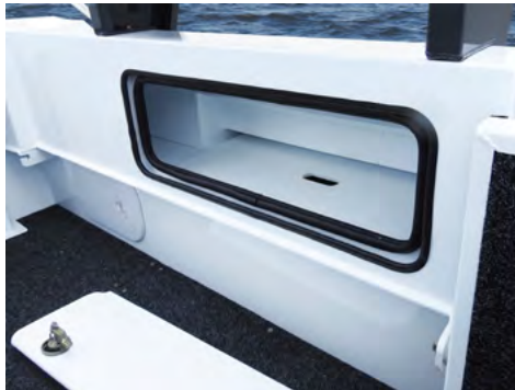
Formosa SRT™ Transom Storage with on-board battery access.
