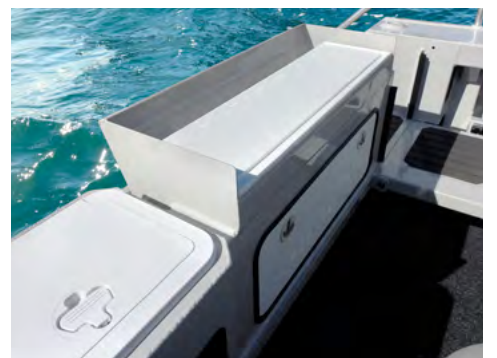
OPTIONS: Live Well with viewing window and hatch. Low Profile Bait Board with custom rod holders.
