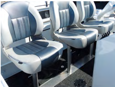
Three folding seats and pedestals with six seat positions in total.
