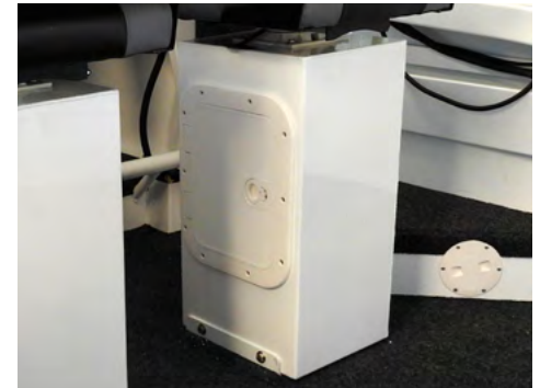
PRO DECK™ Aluminium Self-draining deck has aluminium seat boxes with hatches.
