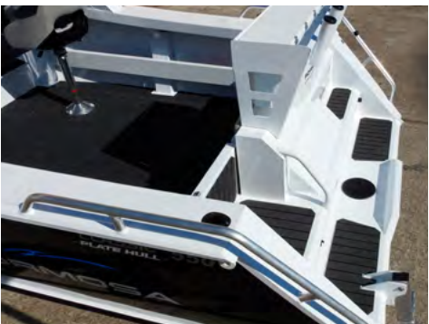
Single Access 'Active Transom' is standard with flush folding transom door. Step down transom, internal grab rail, heavy-duty dive ladder.
