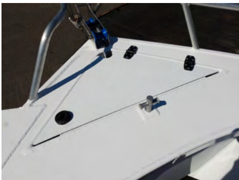
STANDARD: Bowroller, 32mm hand rails, electric motor mount, aluminium anchor well and bollard. OPTION: Anchor Well Hatch.
