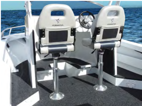
Forward raised casting deck. Air Ride Adjustable Pedestals with folding seats.
