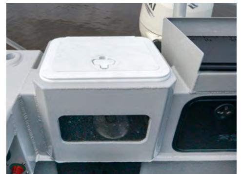
NEW OPTIONS: Transom Live Well with viewing window and Low profile Bait Board (rod holders optional on bait board).
