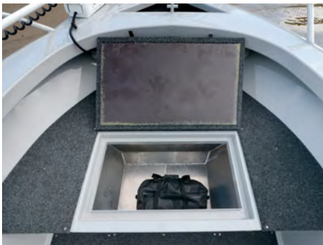
Casting deck storage with drainage system and room for a 70L icebox underdeck.
