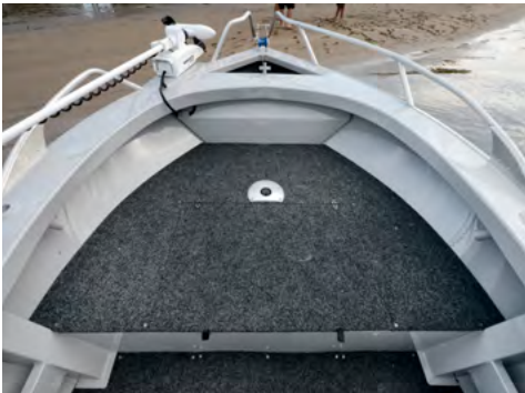
Raised casting deck with enough room for icebox storage underfloor for more deck space.
