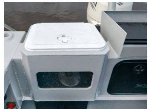
NEW OPTIONS: Transom Live Well with viewing window and Low profile Bait Board (rod holders optional on bait board).
