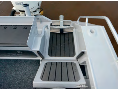
Folding transom door with S/S latch, heavy-duty folding transom ladder and grab rails. Aluminium rod holders on gunnels.
