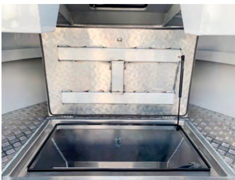
Large storage bay shown with aluminium raised deck.
