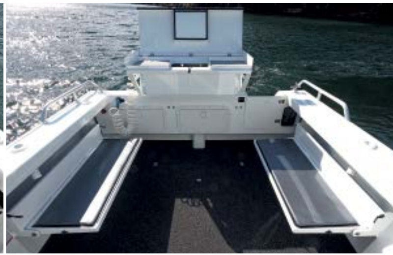
The cockpit's high sides provide support when fighting fish in rough conditions, and metal seats along both sides fold down for use, revealing hidden storage pockets.
