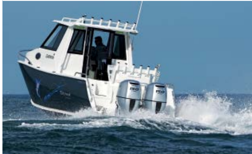
The pair of Honda 150hp 4-strokes delivered a quiet ride with a top speed of 71kph (38kts) and a range of 214km.
