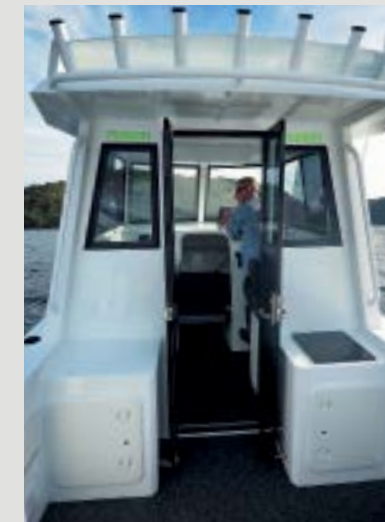
Behind the cabin are storage compartments, a sink with freshwater tap and a 50L slide-out Waeco 12v fridge. Lockable bi-fold doors secure the fully enclosed cabin with wrap-around glass windows.
