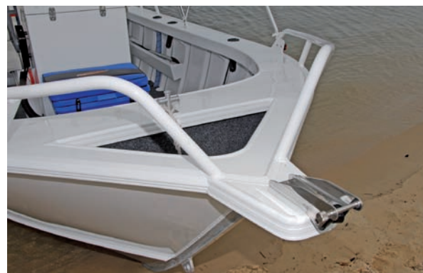
The Formosa's deep anchor well is serviced by a large bowsprit and bow roller.
