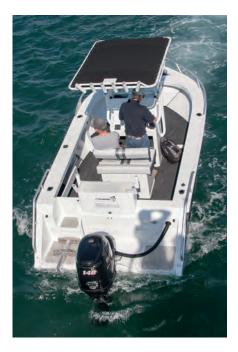
520 Tomahawk is about 1260kg, or comfortably within the tow range of the Toyota Kluger (2000kg), Subaru Outback (1500kg) or new Jeep Cherokee (2270kg). Certainly, she will be a boat suitable for under-cover parking because the Tee-top folds down at dash level.
