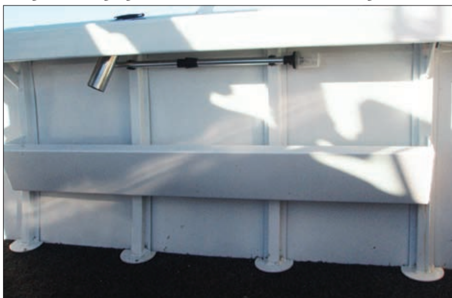
Ample ribbing on the Formosa gives good hull strength.
