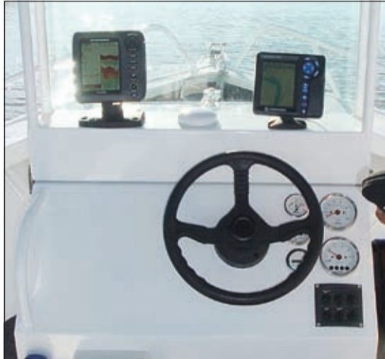
The centre console has plenty of room to either flush mount or top mount the electronics.
