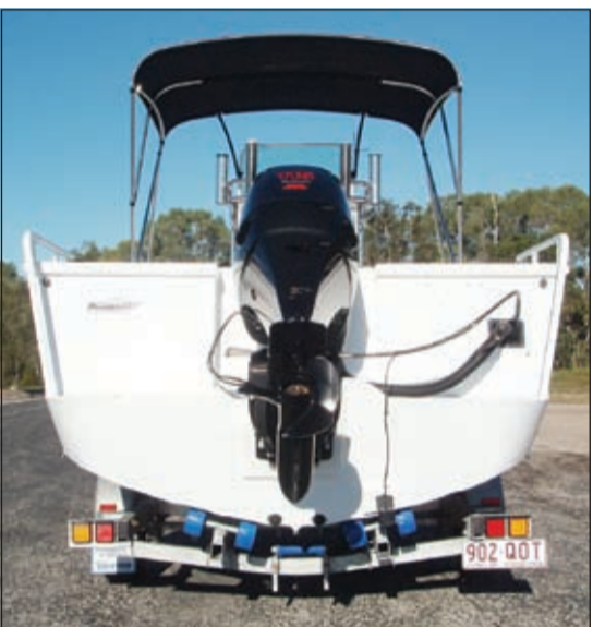
The rear view shows a clean and functional transom with a 15-degree deadrise.
