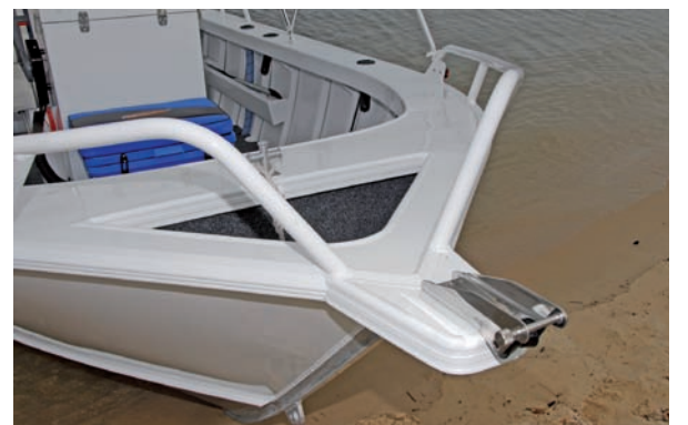
The Formosa's deep anchor well is serviced by a large bowsprit and bow roller.
