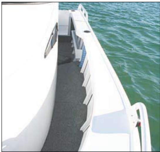
The walk around cab provides easy access to the bow of the boat. Note the amount of ribs making this a solid hull.
